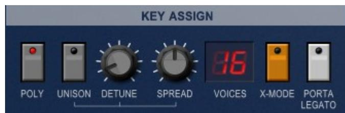
X-MODE is a special performance mode where the enabled oscillators are played in sequence per key (in contrast to all at the same time). For example if oscillators 1 and 2 plus X-MODE are enabled, the first note pressed will cause only oscillator 1 to play while the next note plays oscillator 2 etc. This way you can produce very different sounds per note.
