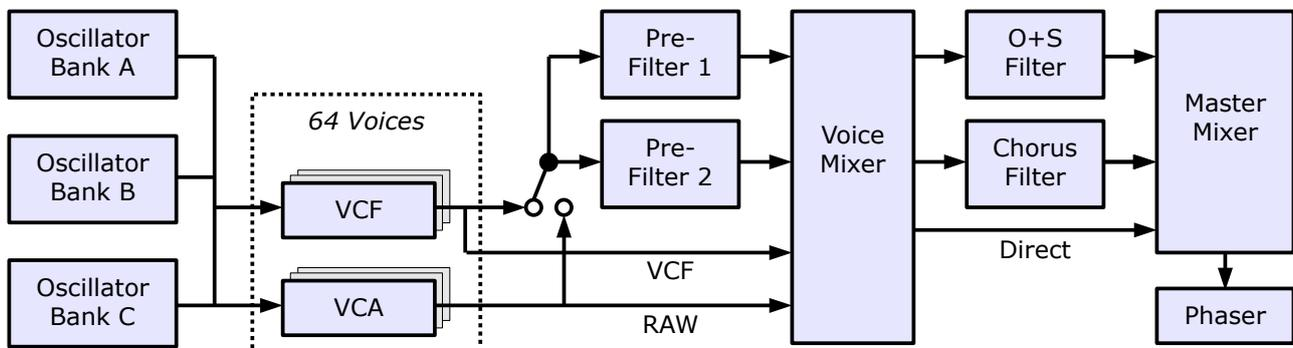
Note that the four separate fixed one-pole lowpass filters of the *PE-2000* for the four "Organ" and "Strings" presets are combined in the O+S Filter of the *PECS*.
