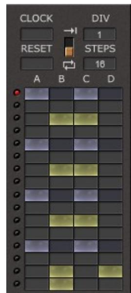
The *Beat Sequencer* module has nine trigger outputs: *Clock*, *Clock Div*, *Clock Link* (clocks only in non-looping mode when the sequencer has finished the last sequence step), *Reset* (clocks when the sequencer resets to step 1), *Stop*, *Line A-B* (clocks for the individual sequencer lines).
