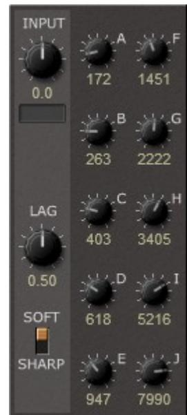
The *Analyzer* module has ten modulation outputs (one per frequency band).
