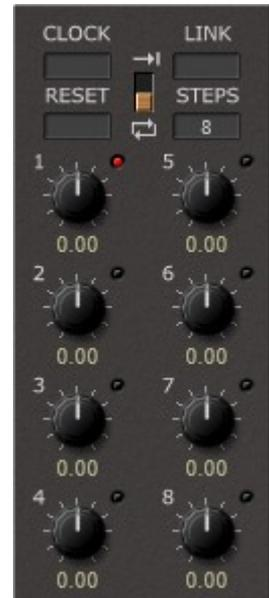
The *Sequencer* module has one modulation output and twelve trigger outputs: *Clock*, *Clock Link* (clocks only in non-looping mode when the sequencer has finished the last sequence step), *Reset* (clocks when the sequencer resets to step 1), *Stop*, *Step 1-8* (clocks for each individual step).
