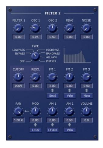
the input of the filter stage. If *Resonance* is set to a value near 100 the filter will start to self-oscillate.
