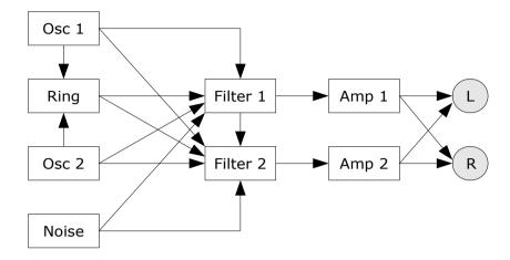
Each voice of the *blooo* features two oscillators feeding a Ring modulator. The individual outputs of the oscillators, the Ring modulator, and an additional white noise generator are sent to the input mixers of two multi-mode filters; furthermore, Filter 2 can receive the output of Filter 1. The filter outputs are routed to two individual amplifiers with panorama control which are connected to the main stereo output bus.
